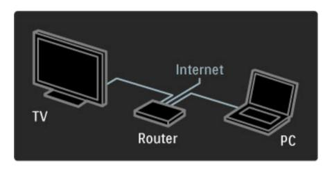
If you use a wired connection to the router you need a network (Ethernet) cable.
